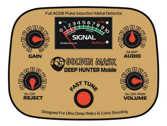
"**VOLUME ON/Off**" - knob to switch "ON/Off" the detector and adjusting the level of sound.
